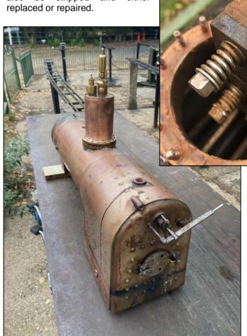
Once these issues have been resolved the process of attaching all the fittings will be possible. Then a hydraulic test can be arranged.
